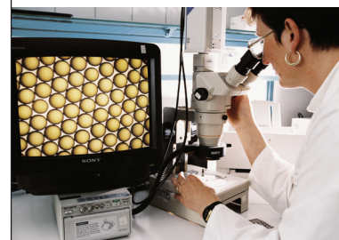
Figure 4: Ion exchangers are made of microscopic polymer beads with specific chemical properties: Quality check in an application test laboratory at LANXESS Deutschland GmbH
